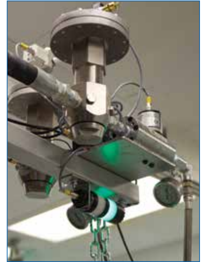
The green light on the ExactaBlend AGP system indicates that materials are being applied properly and on-ratio.
