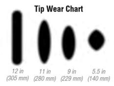
If using a worn tip, on average you will spray 25% more paint and 20% in additional labor.
