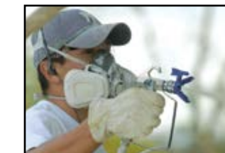
FTx 4-finger gun trigger – full length trigger is easier to hold in continuous spray.
