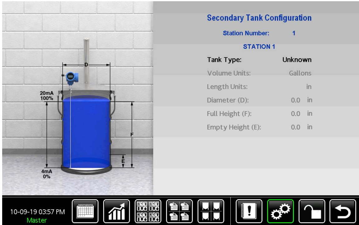
Figure 74 Secondary Tank Configuration Screen
