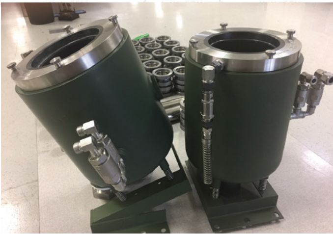
Bell Washer Optimization Project to reduce spray defects from Bell and increase time between housekeeping and service intervals, plus tool free connections for the blow off ring.
