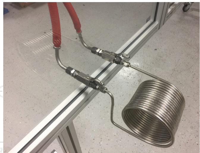
Pre-Constructed, cleaned and ready to install Restrictor Station to simulate pressure loss in an active station to keep the flow and pressure in balance in a paint circulation system.
